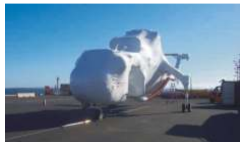
Under-Raps™ N.S.W wrapped Sikorsky 58T for shipping as deck cargo protected in Intercept shrink film.
