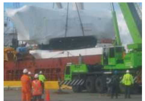
Under-Raps™ N.S.W wrapped Sikorsky 58T for shipping as deck cargo protected in Intercept shrink film.
